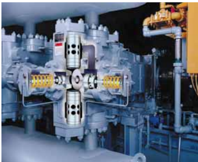
A cutaway view of Dresser-Rand's Storage Cylinder.
