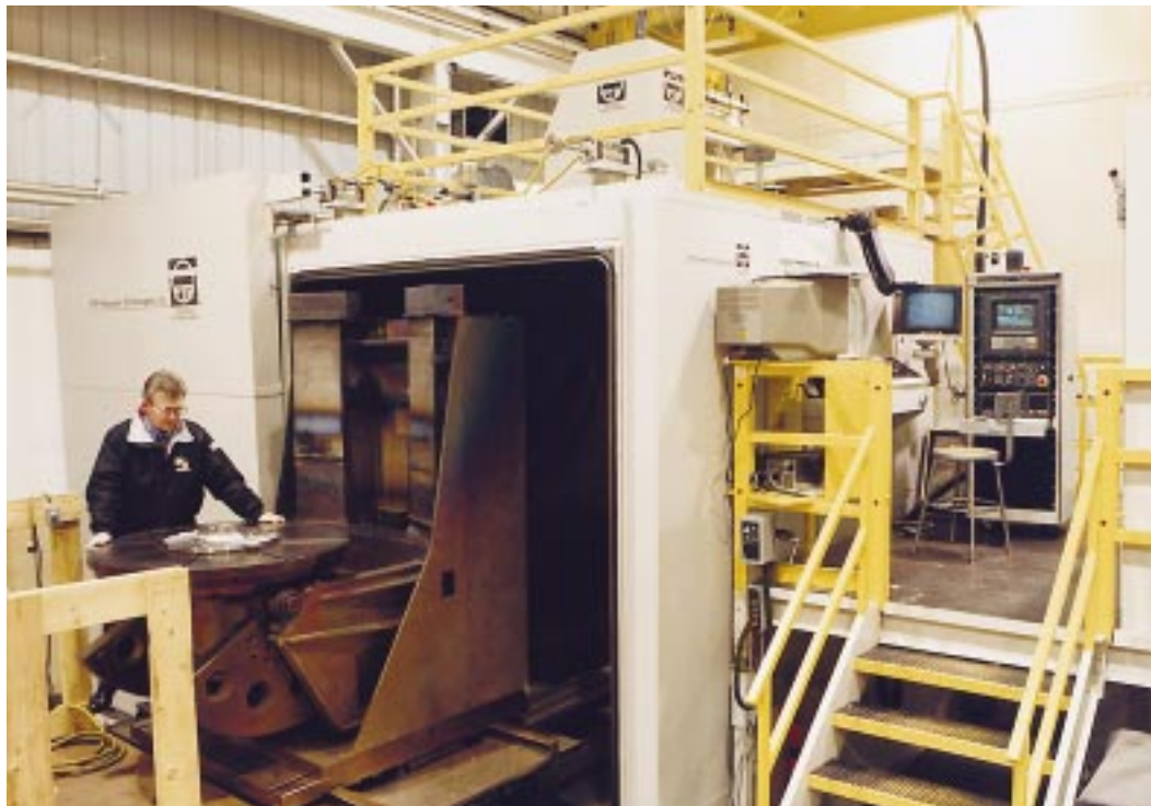
Dresser-Rand's new electron beam weld machine can accommodate the largest impeller in the DATUM line of centrifugal compressors.
